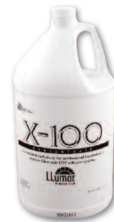
GT714 X-100 APPLICATION SOLUTION- GALLON Cleaning and application concentrate for most dry adhesives. The mild acid formulation makes this a great cleaning agent for glass contaminated with oil, grease or dirt. Recommended mixture is 1 ounce per 1 quart of water. Not to be used with copper or silver based films.
